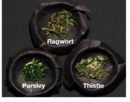
In this example Headwall's Hyperspec<sup>®</sup> MV.X system is used to identify ragwort in a mix of parsley and thistle herbs. A spectral classification method was developed using a sample of each plant as a reference. The method was then tested on two samples, containing ragwort intermixed with other herbs. Images on the left show the individual samples and it is easy to see how challenging sorting them could be using traditional vision.
